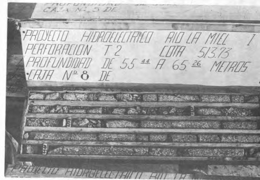
CORE FROM BORING T-2 THROUGH THE CONTACT OF SCHIST AND QUARTZ-DIORITE
