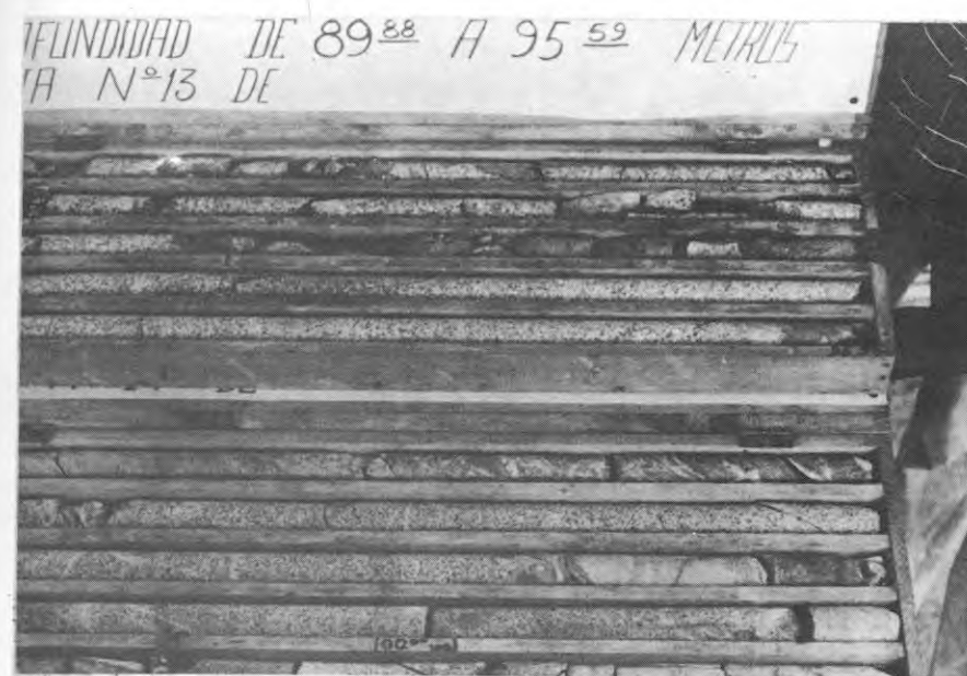
2 - FRESH QUARTZ DIORITE AT 90 TO 100 METERS DEPTH IN T-2
