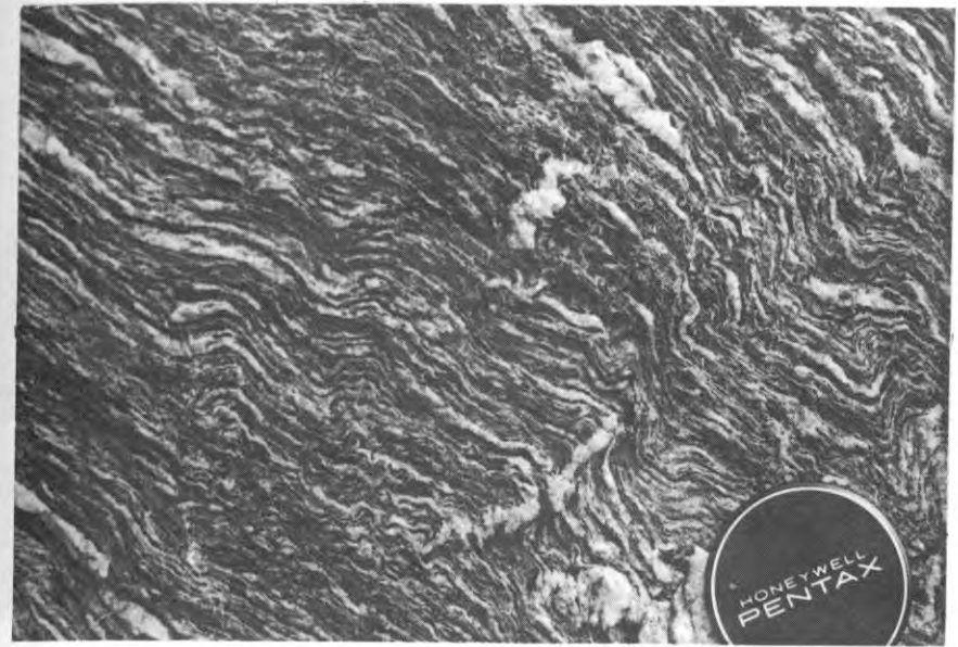
CRENULATED SCHISTOCITY AT THE MIEL I DAM SITE
